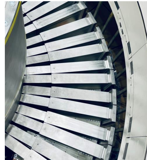
Port tubes after welding 2.9 mm (lateral)
